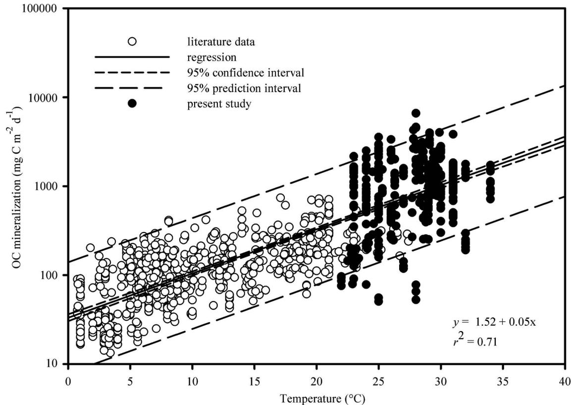
Fig. 5. The relationship between sediment OC mineralization rates and temperature in lake sediments. Data include values from the literature ( $r^2 = 0.43$ ,  $p < 0.0001$ ,  $n = 574$ ; Gudas et al. 2010) and the present study ( $r^2 = 10$ ,  $p < 0.0001$ ,  $n = 392$ ). The regression for the two combined data sets is shown ( $r^2 = 0.71$ ,  $p < 0.0001$ ,  $n = 966$ ). The  $y$ -axis of OC mineralization rates is represented on a log scale.
