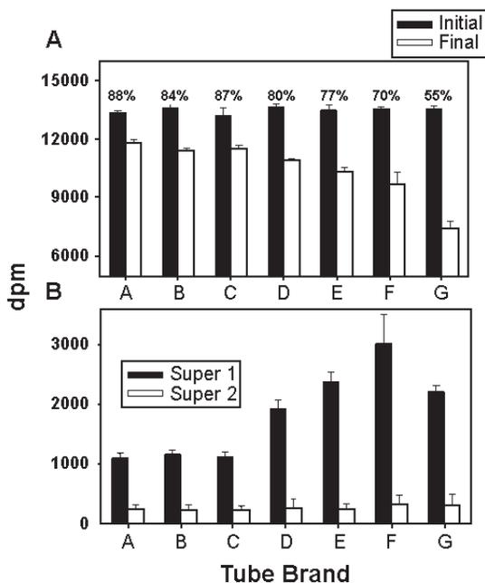
**Fig. 3.** Protein retention in different tube brands. (A) Comparison of initial and final disintegrations per min (dpm) and (B) dpm lost in the supernatant of the first and second trichloroacetic acid washes. Values are means  $\pm$  1 standard deviation.
